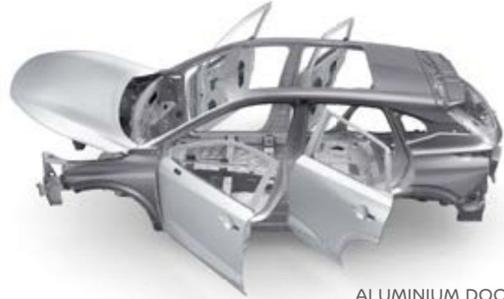
ALUMINIUM DOOR PANELS AND BONNET Lighter aluminium panels in the door and bonnet help reduce weight and therefore CO 2 emissions.
